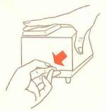
OPENING AND CLOSING CASE: Grasp projector with right hand. With left thumb, press down gently on metal latch near bottom of Case Back, at the same time lifting Case Back out and up with right hand. To close, set the Case Back at a slight angle against Case Front, tops together. Swing Case Back down into position, snap shut.
