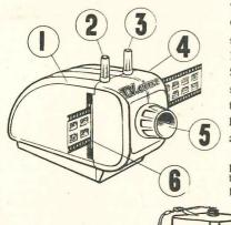
TO LIGHT UP THE PROJECTOR LAMP, connect the **T.V. CINE** to a LANTERN BATTERY (Ever Ready R 996 or any similar make) If it is to be operated from the mains, use the MINICINE TRANSFORMER as explained below.
