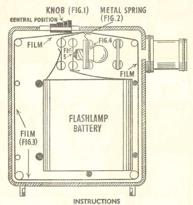
To Open Projector slide Knob to central position of slot as shown in diagram, Fig. 1.
