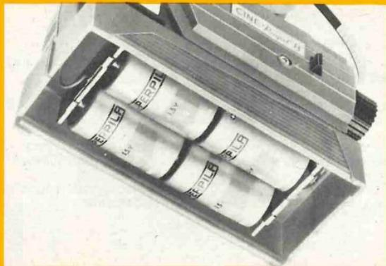
1. The functioning of the unit is given by four 1,5 V batteries.
